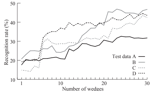
Figure 7: Experiment 3: Recognition rate and number of wedges per hand type and palm direction (person is unknown).
